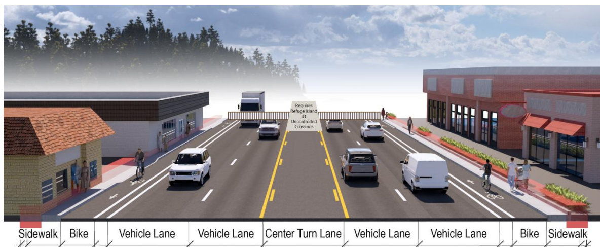
Figure 6. Central Segment Alternative 1 – Five Lanes (Facing South)
